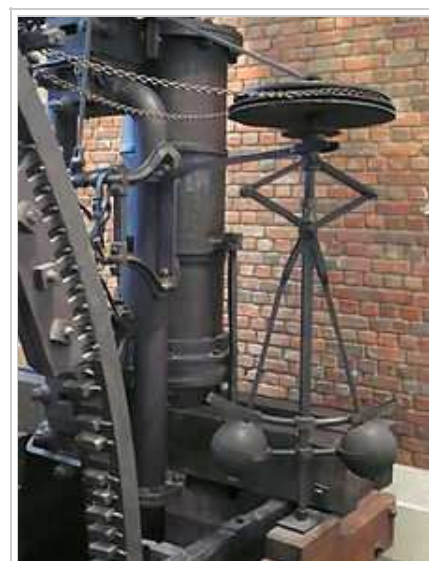
Centrifugal governor in a Boulton & Watt engine of 1788
