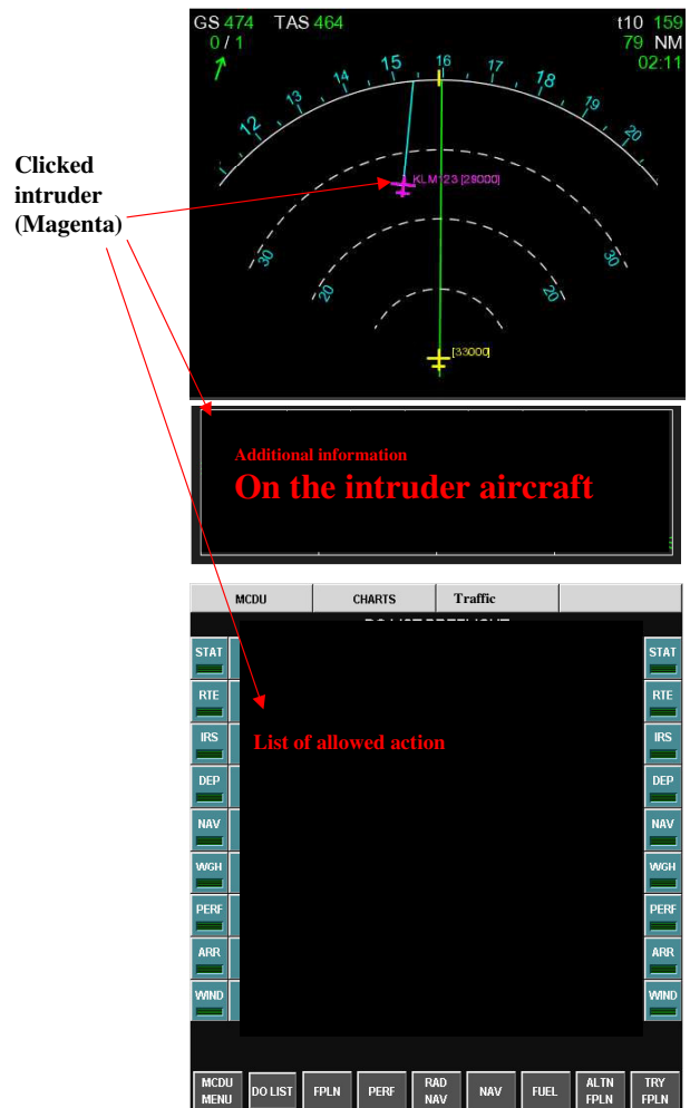
Figure 2 illustrates that a service is executed by clicking on an object in the Navigation Display. That service gives additional information related to the object in the vertical window, plus associated actions in the window of the MCDU. The information and further actions that are shown are a property of the service. The location of the service is transparent to the users, and herewith the functionality of the service might depend (if specified) from the actual service that is used. E.g. a TIS service provided by an airport may provide different functions from a TIS service for en-route. The services will then propose different user interfaces.
